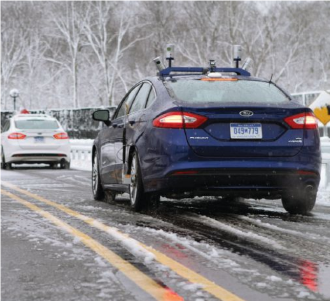
Ford’s autonomous vehicles employ high-resolution 3D mapping and LIDAR to facilitate driving in bad conditions when road markings aren’t visible. Image courtesy of Ford.
