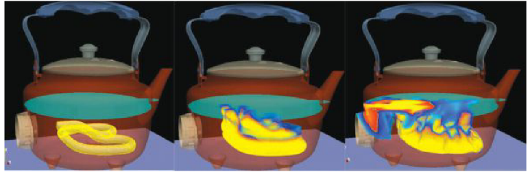
CFD solver is coupled to the solid thermal solver and the Electro-magnetic solver to simulate the heating of water inside an electric kettle which is plugged into a standard 110V switch.
