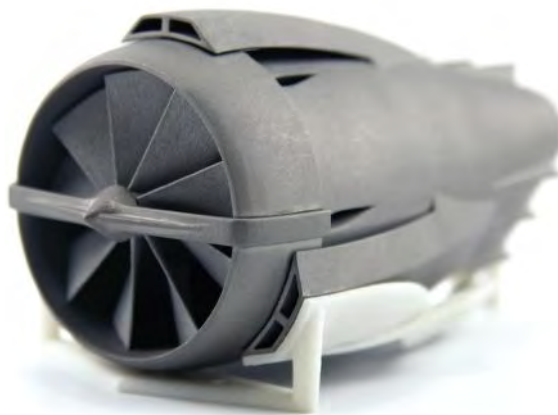
PolyJet technology is capable of creating multiple materials and colors in a single print. Image courtesy of Stratasys.
