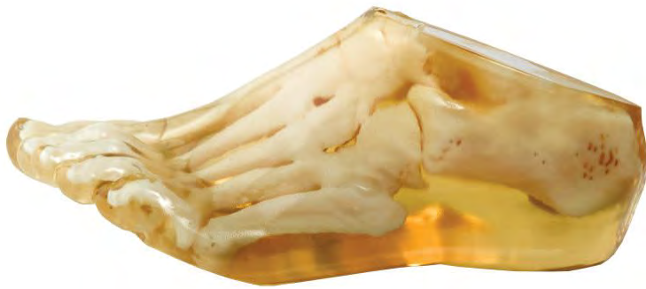
PolyJet technology is capable of creating multiple materials and colors in a single print. Image courtesy of Stratasys.
