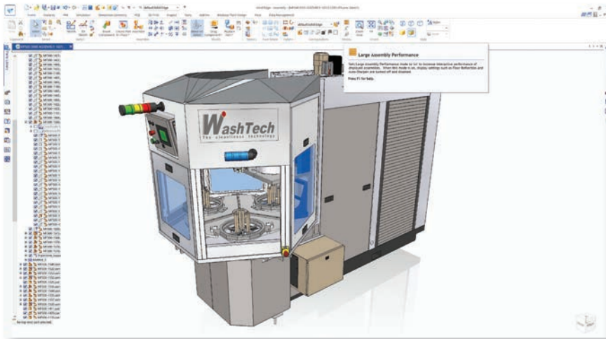
In rotating large assemblies and selecting components, the GPU-rendered visuals impact real and perceived software performance. Image courtesy of Solid Edge, Siemens PLM.
