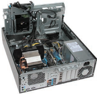
An exploded view of the HP Z2 SFF G4 workstation. Image courtesy of HP.
