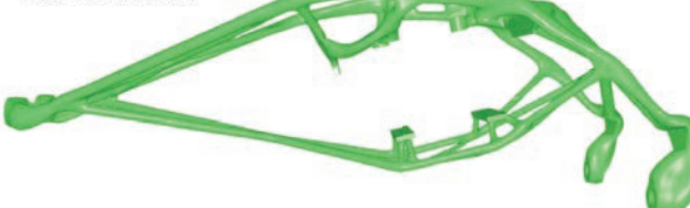
FIG. 9: Configuration minimizing compliance under varying stress constraints.
