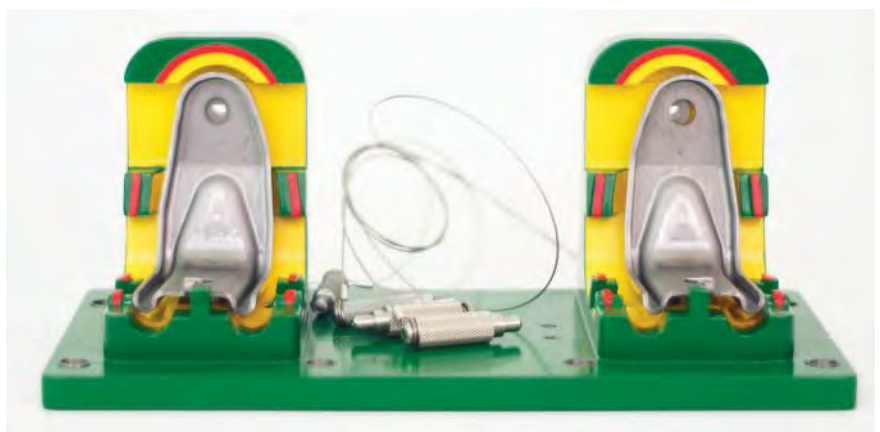
An original aluminum fixture (top) and a 3D printed iteration (bottom) with clamp-on assemblies. Images courtesy of Stratasys Direct Manufacturing.
