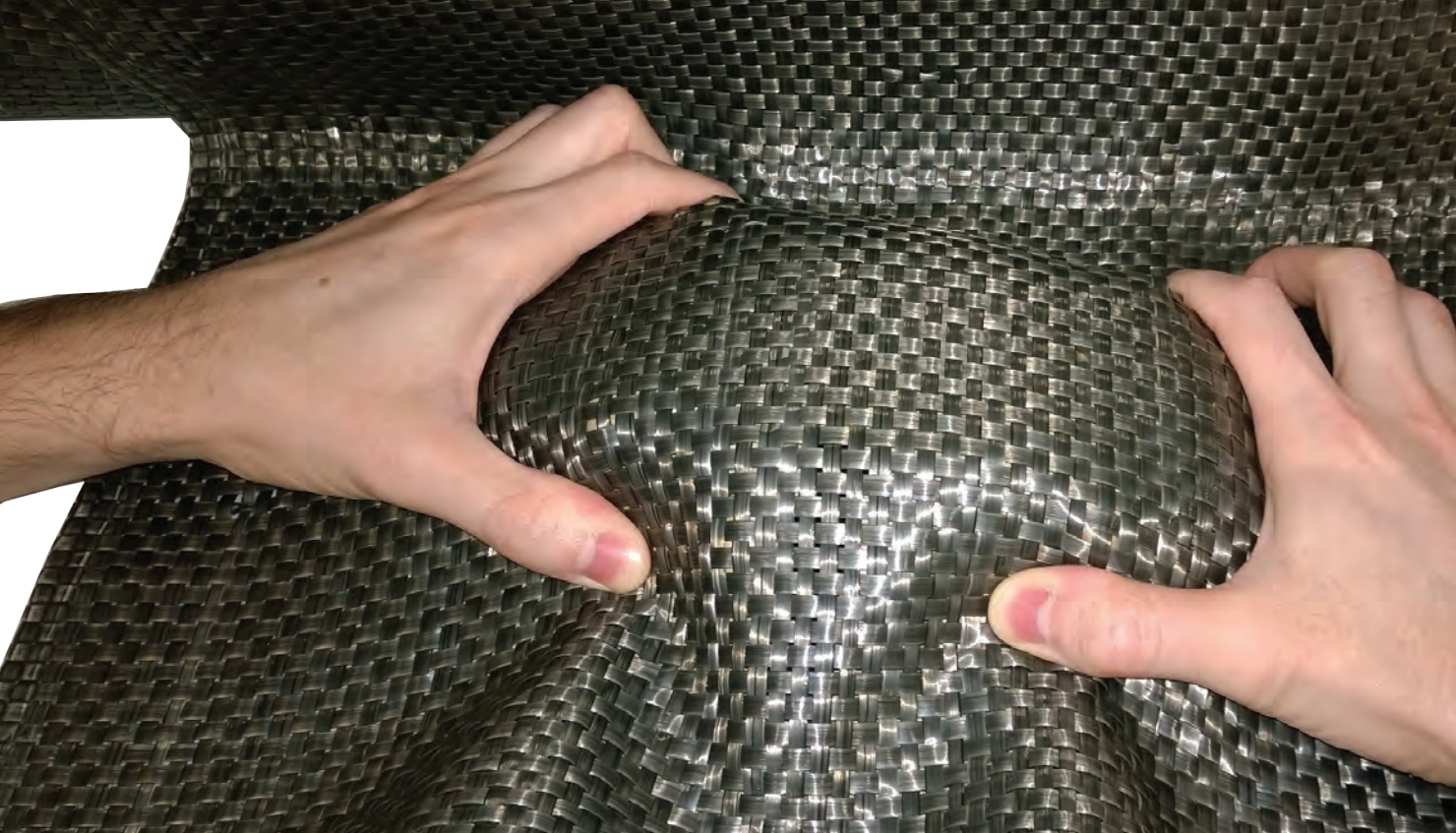
A cover made from Fibrtec's Fibrflex prepreg (left) and an image showing the drapability of Fibrflex over the cover mold. Images courtesy of Fibrtec.
