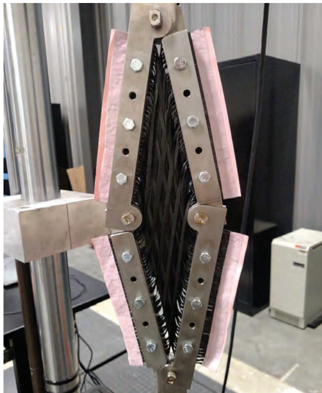
DuPont's Rapid Fabric Formation technology deploying Fibrflex at high shear angles. Image courtesy of the Institute for Advanced Composites Manufacturing Innovation.
