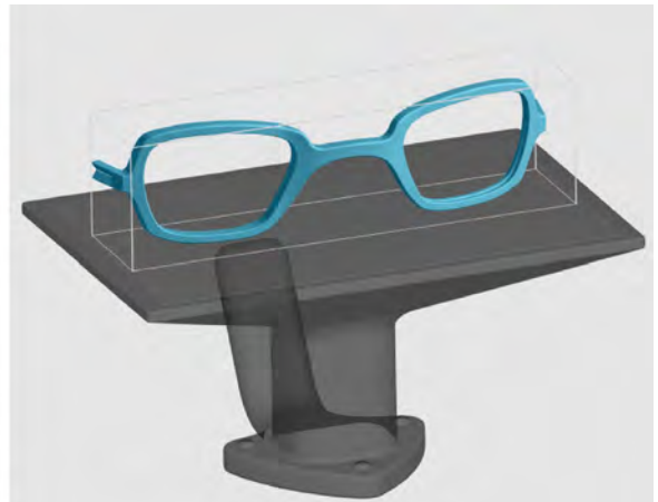
Loving Eyes Foundation uses magnetic resonance imaging and computed tomography scan to reconstruct a patient's head, then 3D-print custom eyeglasses. Image courtesy of Carbon.
