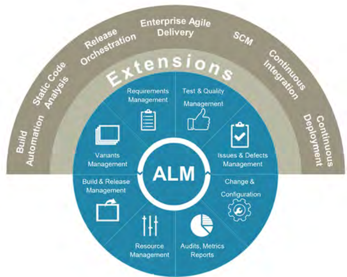
Fig. 2: Application lifecycle management (consists of an amalgam of functions tailored not only to meet the unique demands of the software development process, but also to facilitate collaboration, speed software development and improve testing. Image courtesy of Siemens Digital Industries Software.
