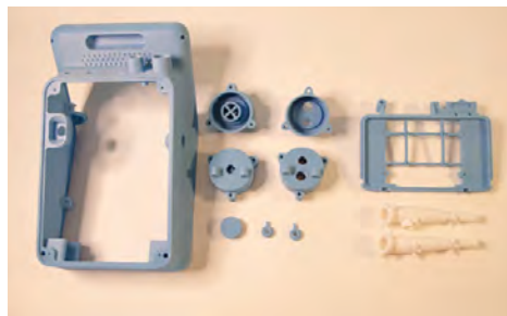
InVent Pneumatic Ventilator prototype parts from a Stratasys J850 3D printer.
