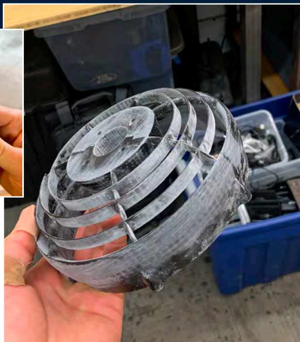
The printed prototype parts are durable enough to withstand multiple rounds of in-water testing. Images courtesy of 3D Systems.
