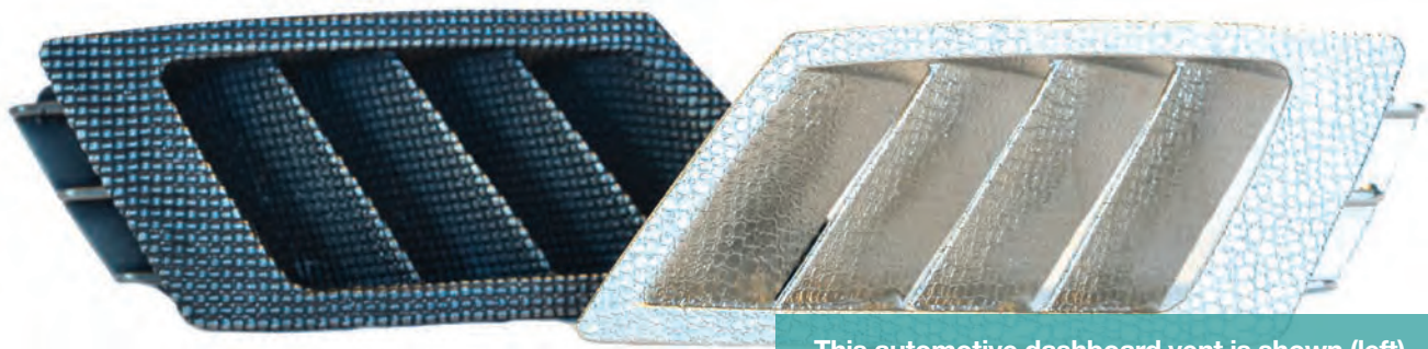
This automotive dashboard vent is shown (left) as the initial piece directly from the Figure 4 production printer and (right) after plating directly onto the part. Image courtesy of 3D Systems.
