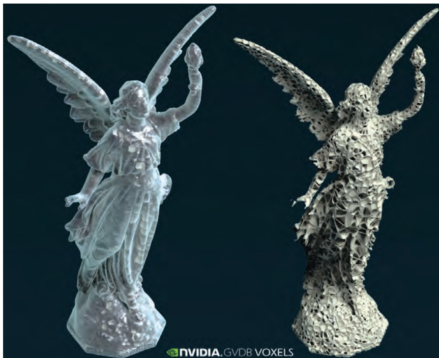
Voxel-based 3D printing with NVIDIA GVDB (GPU voxel database), where the inside structure is optimized based on stress and automatically generated. Image courtesy of NVIDIA.
