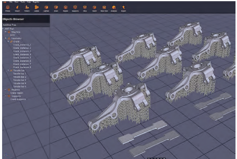
Dyndrite uses CPU and graphics processing unit (GPU) computational power to streamline model preparation for additive manufacturing. Image courtesy of Dyndrite.
