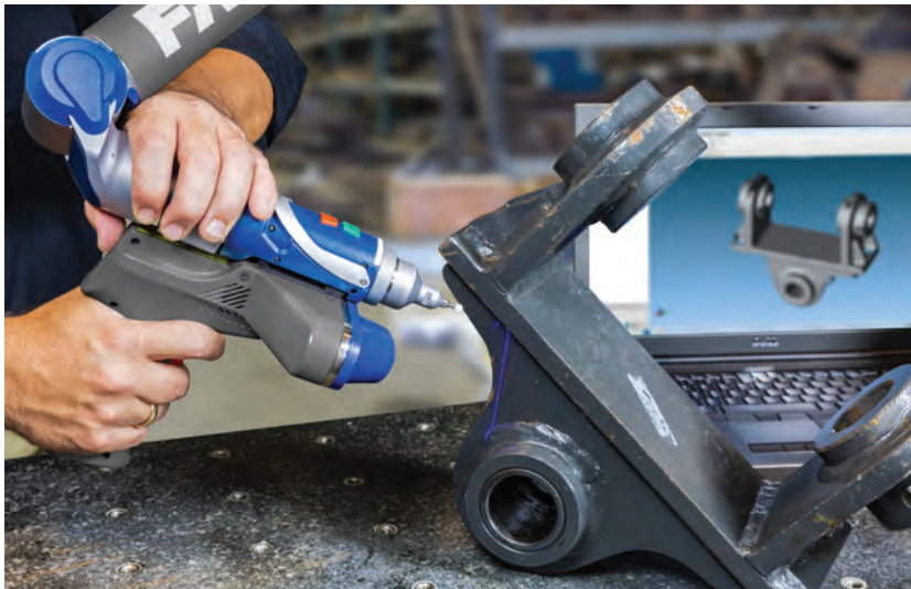
Hard probes and touch probes provide more accurate results than non-contact scanners, but at the expense of speed. Image courtesy of FARO.
