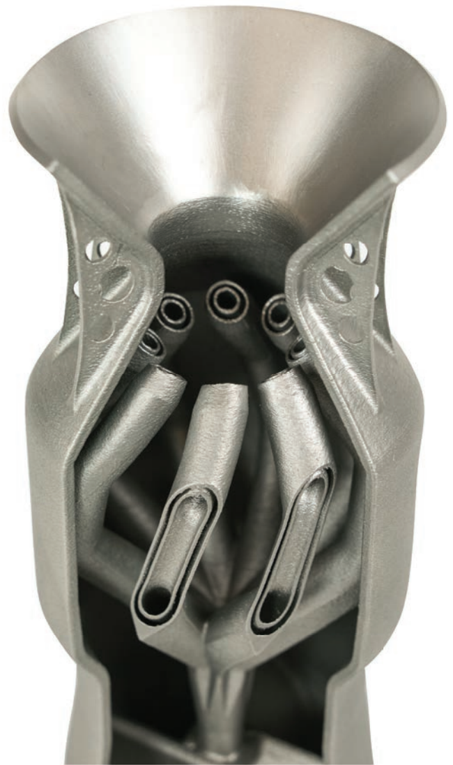
Fuel nozzle printed on 3D Systems’ ProX DMP 320 in LaserForm CoCrF75(A) for high corrosion, wear and high temperature resistance. Image courtesy of 3D Systems.
