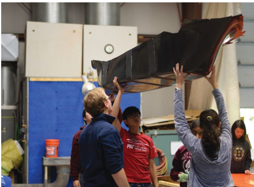
Key to the MIT Flux's lightweight design is a new carbon fiber shell and chassis. Image courtesy of MIT, Micah Gale '18.
