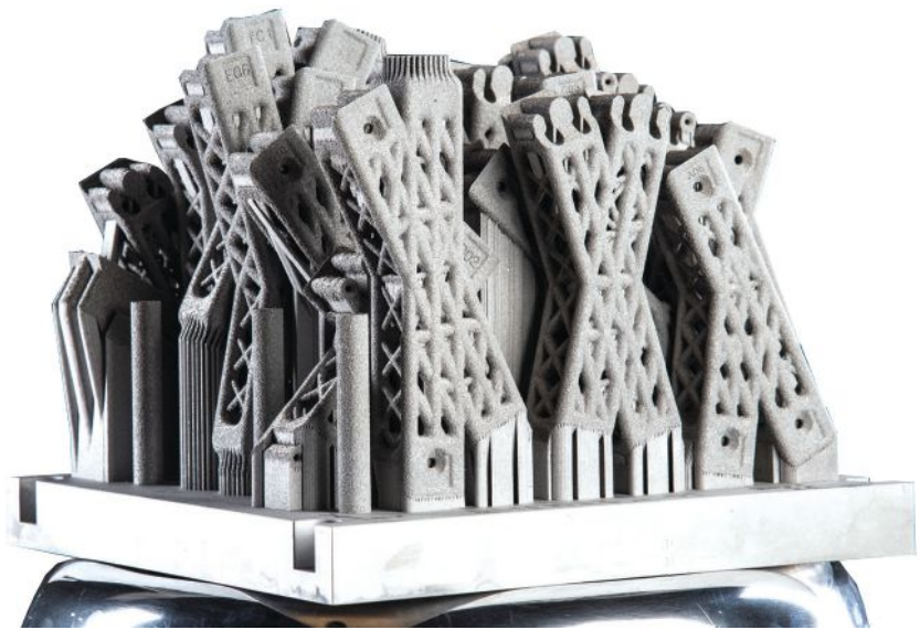
The bionic partition, which separates the seating sections in an airplane, is designed using algorithms that mimic slime mold behaviors. Image courtesy of Autodesk.
