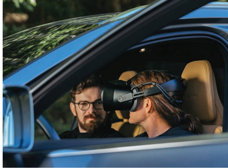
A test driver for Volvo wears a Varjo XR-1 AR headset to see the virtual dashboard of a new model under development. Images above and opposite courtesy of Varjo and Volvo.
